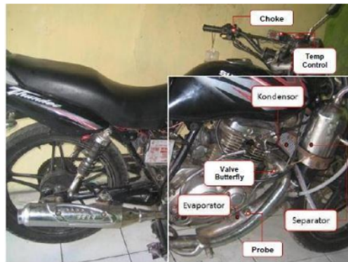
FIGURE 1. Experimental Set up on Motorcycle
