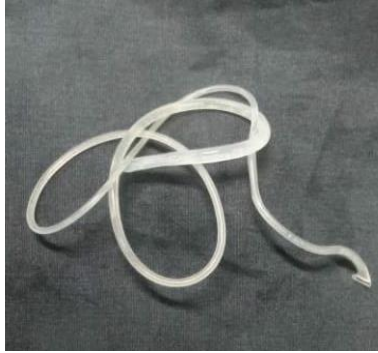
FIGURE 4. Melt flow rate result of as received specimen
