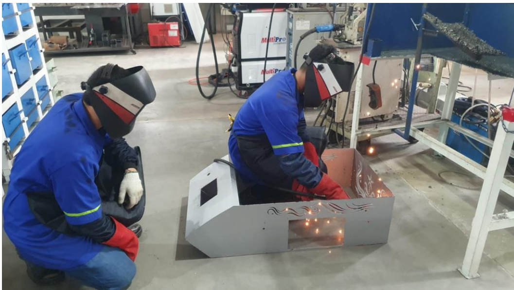
Gambar 11. Proses Welding cover Body AGV
