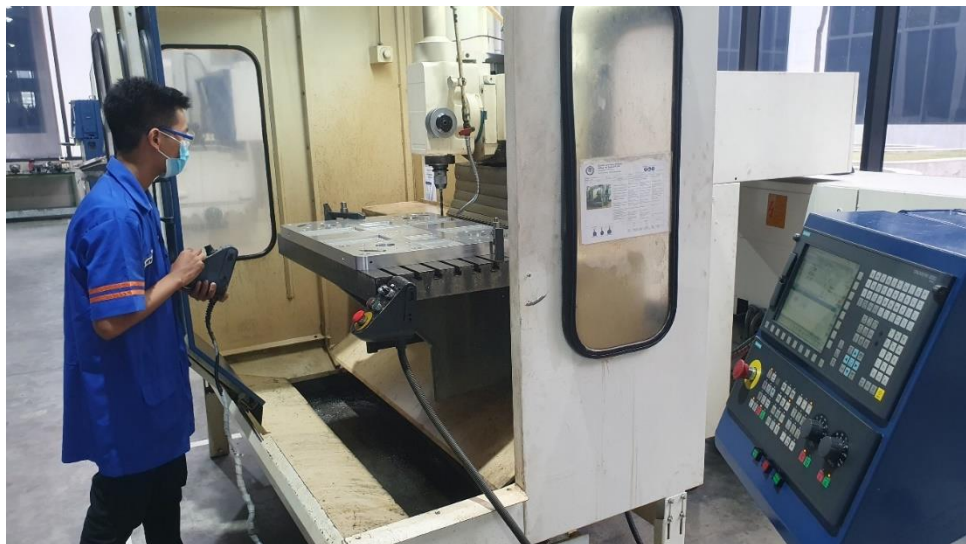
Gambar 9. Proses Machining Chassis Aluminium di Mesin CNC-Milling
