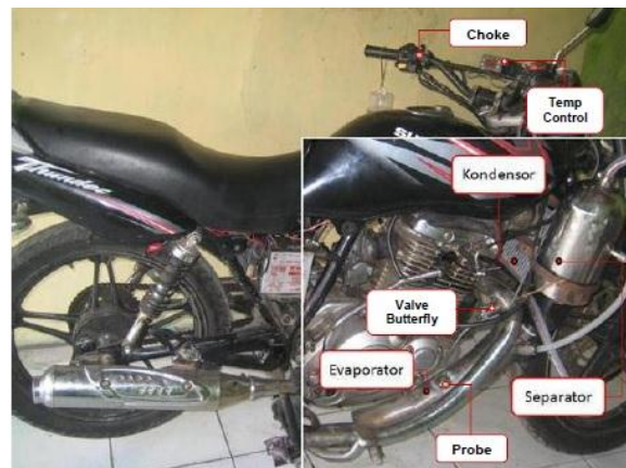
FIGURE 1. Experimental Set up on Motorcycle
