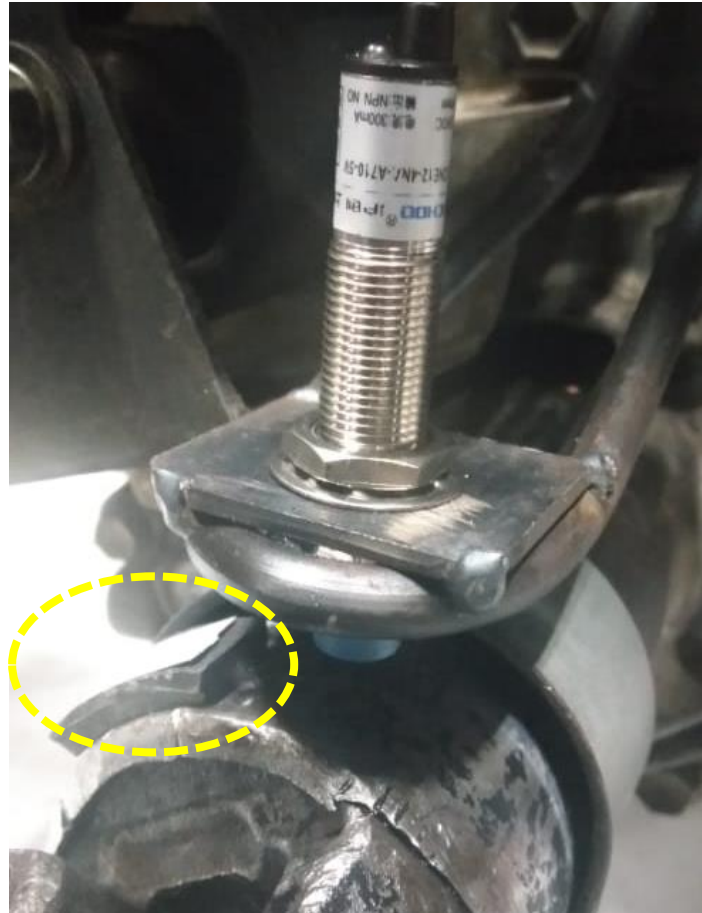
Figure 65. Iron blade to trigger Signal
