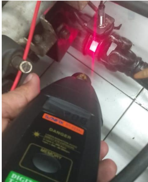
Figure 57. Validation With Tachometer
