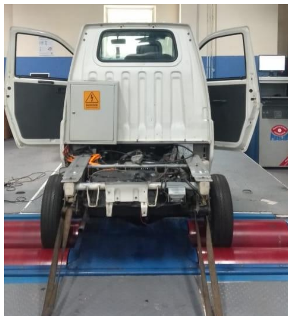
Figure 28. Performance test on Dynamometer (2)
