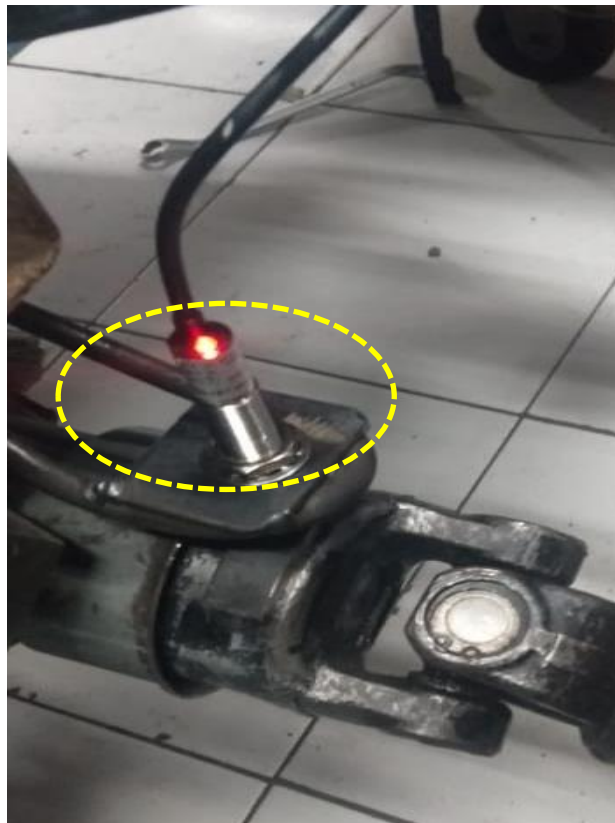
Figure 64. Inductive Proximity Sensor on top of the Propeller Shaft
