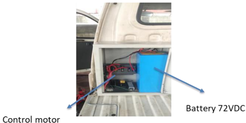
Figure 5. Battery and Control Motor
