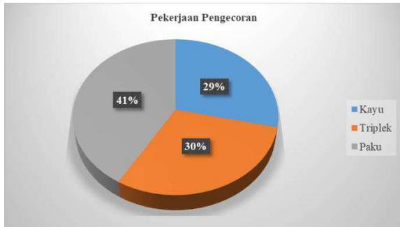
Gambar 5. Diagram Persentase Sisa Material Pekerjaan Bekisting
