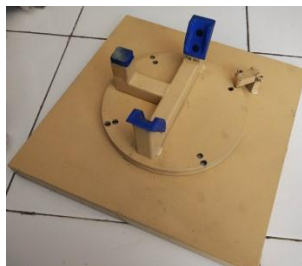
Gambar 5.12 Fixture Holder Part PP Grip
