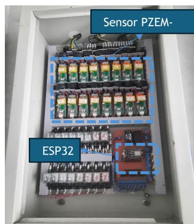
Gambar 6. Panel Utama Laboratorium Mekatronika
