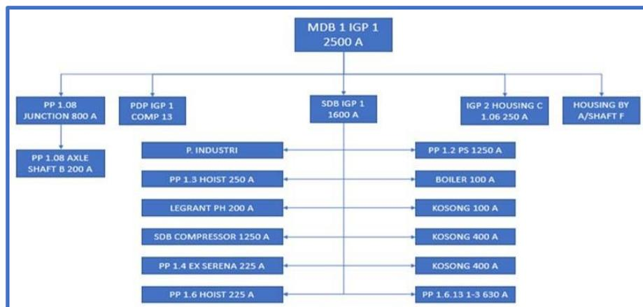
Figure 1. The electrical distribution diagram of MDB 1
