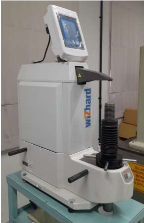
Gambar 2. Alat Uji Kekerasan Material Wizhard HR-522
