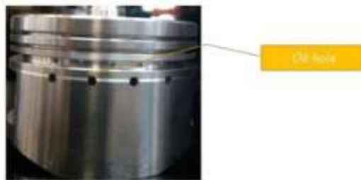
Figure 2. Oil hole drilled by DOH machine.
