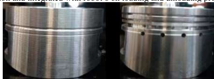
Figure 15. Result of drilling from DOH machine
