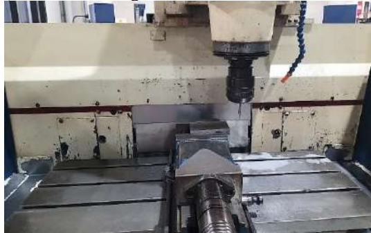
Figure 5. Machining Setup and CNC Milling Makino KE-55
