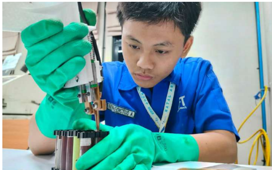
Gambar 11 Proses Spot Welding Battery Pack
