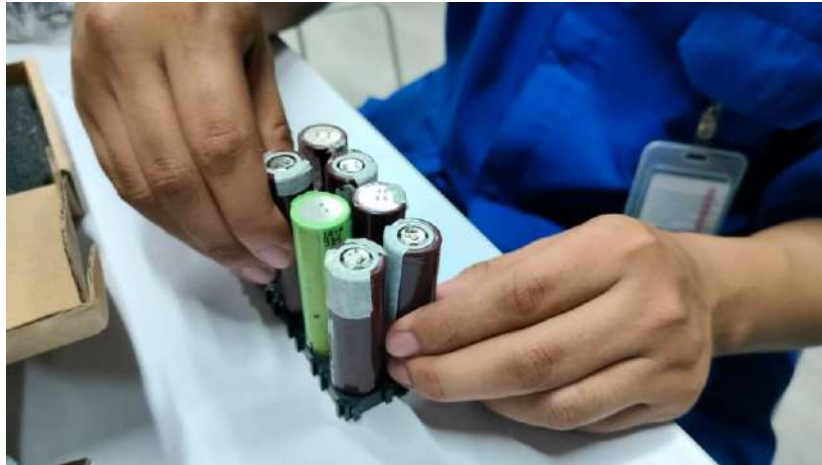
Gambar 10 Perakitan Battery Pack
