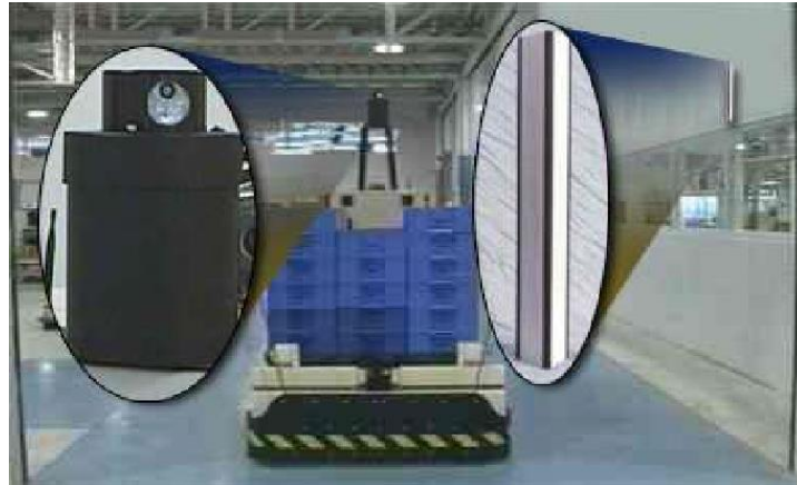
Gambar 2.9 Laser Guided Vehicle
