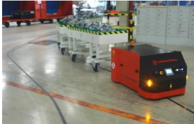
Gambar 2.8 Magnet Guided Vehicle
