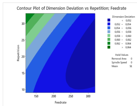
Figure 7. Contour Plot of Dimension Deviation on S-33 Machine.
