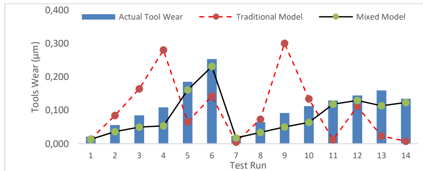
Fig. 1. Wear of Cutting Tools Response Value and The Proposed Prediction Model Result
